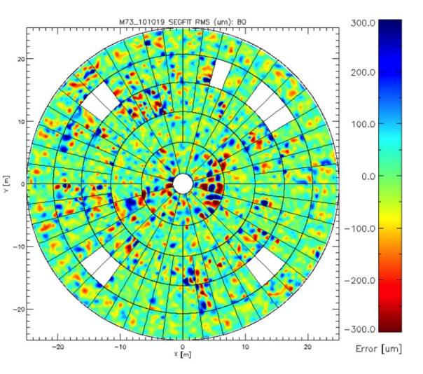
A single surface error map from photogrammetry data.
