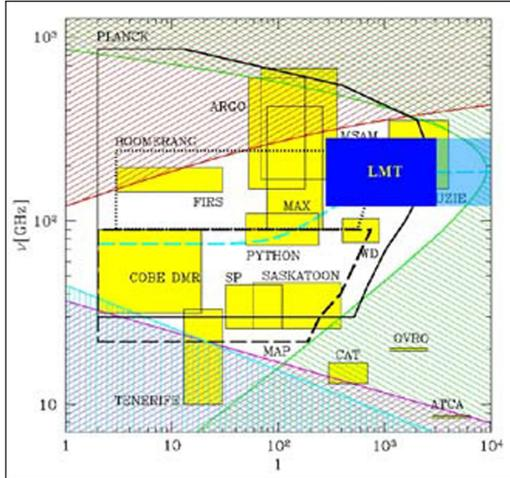
Figure 3.11 Telescope sensitivities as a function of angular scale ( $l \sim 120$  /deg) and observing frequency. The opaque LMT region represents the practical limits with its initial instrumentation. The extended transparent blue region would be possible with future generations of 1000+ pixel bolometer arrays, given the spatial resolution afforded by the 50 m aperture<sup>24</sup>.
