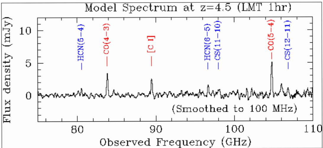
Figure 3.6 Simulated spectrum of a  $z = 4.5$  mm galaxy after one hour of observation using the Redshift Search Receiver on LMT, assuming a system temperature of 100 K. The flux density of CO lines is based on measured line strengths of the  $z = 4.4$  quasi-stellar object BRI 1335-0417. The brightness of other lines is based on average relative ratios observed in nearby luminous infrared galaxies<sup>11</sup>.
