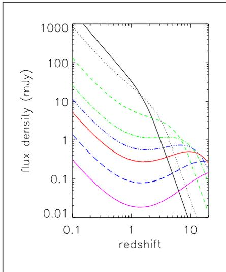
Figure 3.2 (a) The effect of redshift on flux density at far infrared to mm wavelengths for an object similar to the ultraluminous galaxy Arp220. From top to bottom (at a redshift of  $z=0.1$ ) the colored curves show this effect at 160, 250, 500, 850, 1100, 1400, 2100, 3300 microns, respectively<sup>2</sup>.
